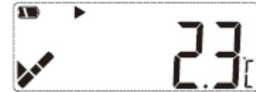
In the example above, the current temperature is 2.3°C and with the tick showing, no alarm conditions have been encountered.
